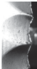
Burr on liner surface
